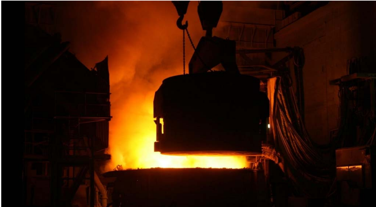
Steel scrap loading into the smelting furnace
